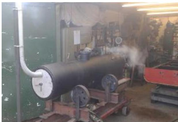
Whilst this was going on our workshop team was working on the tender, fitting the water tank and pipework. New valves were fitted to the cylinder drain taps and a linkage made to connect their operation to the loco cab.
