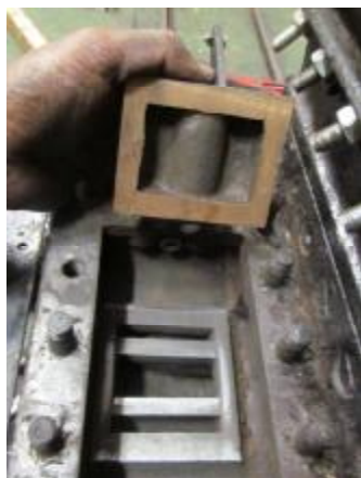
Inside the left hand side valve chest of Railway Queen, with the heavily worn right hand side valve above
