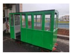
The new Coach 12 now has its bodywork and air brake system complete, It runs satisfactorily on its all-new bogies, but presently we are awaiting the supply of cast brake shoes so that the brake gear can be fitted.
