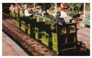
and then later more simple timber seats mounted on the original chassis.
