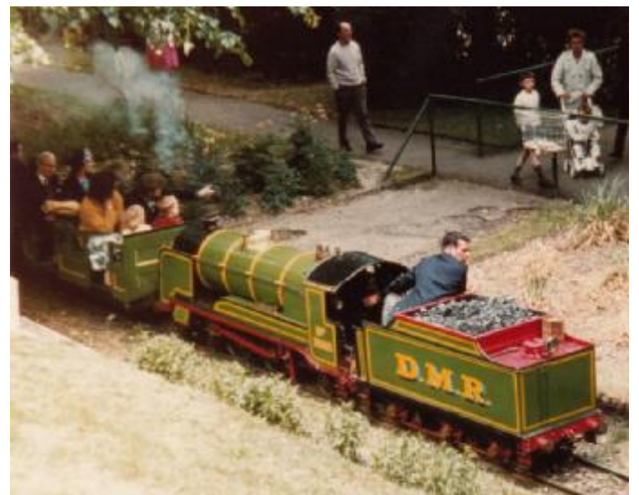
The present boiler carried by Billie was made by Luggs of Billingshurst in 1970. Michael Lugg and his family made a lot of boilers for traction engine owners. Luggs placed mudhole doors on the firebox crown, which are visible here on Billie newly repainted c1971. This boiler also has the dome and safety valve mountings made massively.
