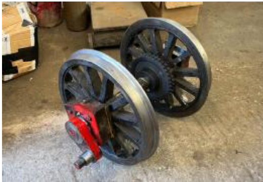
Here is one of the wheelsets, with its tyres re-profiled, bearings renewed and a new drive sprocket fitted.
