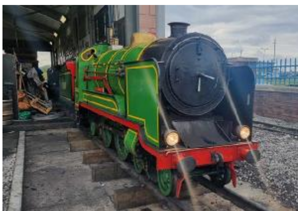
Over the summer Justin completed the cosmetic restoration of Billie by installing working headlights to equip it for night time operation.
